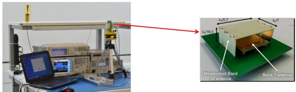
Figure 1: Carrier aggregation demonstrator setup comprising the reconfigurable RF front-end (including a dual band miniature antenna), the control PC and the measurement equipment.
